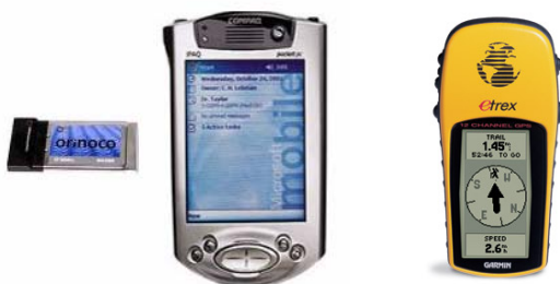
Fig. 4 Equipment used in the test (Wi-Fi card, PDA and GPS receiver)
