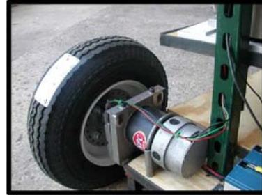
Fig. 9 DC motor and wheel coupling implementation
