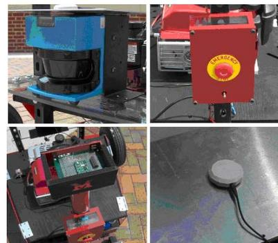
Fig. 14 Specialized mounts: laser ranging system (top left), safety switch (top right), digital compass (bottom left), and GPS antenna (bottom right).
