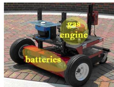
Fig. 10 Power system on the Redblade III
